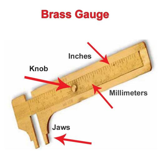
As illustrated, the gauge will give measurements in millimeters and in inches. The bottom row of the gauge provides measurements in millimeters while the top provides measurements in inches.
